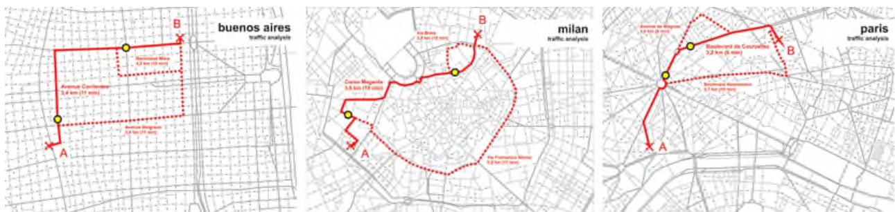
Figure 3: Analysis of alternative routes on selected urban patterns of Buenos Aires, Milan and Paris was performed in relation to the crime prevention through environmental design (CPTED) project. It respects the one-way roads and presents the traffic delay by using the alternative routes. The urban pattern determines the allowed motion. Motivated by G.E. Haussmann for the renovation of medieval neighbourhoods of Paris that were deemed overcrowded and unhealthy, was the quick and easy transportation of forces against public riots.
